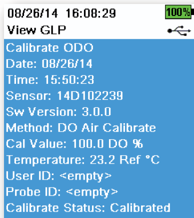
Figure 12 GLP record example (single point % DO calibration)
